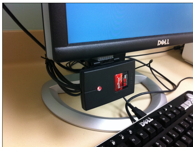
Fig. 1. Photograph of a proximity card reader attached to the bottom of a monitor in one of the patient rooms where the pilot study took place. ID badges brought close (within approximately 5 cm) of the reader activated an automated login process.
